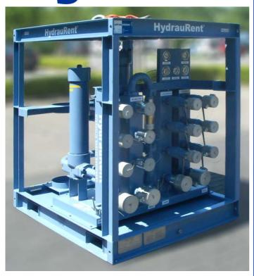
The HydrauSupport 450FF is a multipurpose hydraulic filtration unit and is designed as an additional unit in order to flush piping and to filter hydraulic fluids of hydraulic systems.
