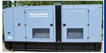
Diesel-driven Hydraulic Power Unit with a maximum engine power output of 391 kW.
