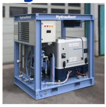
Diesel-driven Hydraulic Power Unit with an engine output power of 34 kW.
